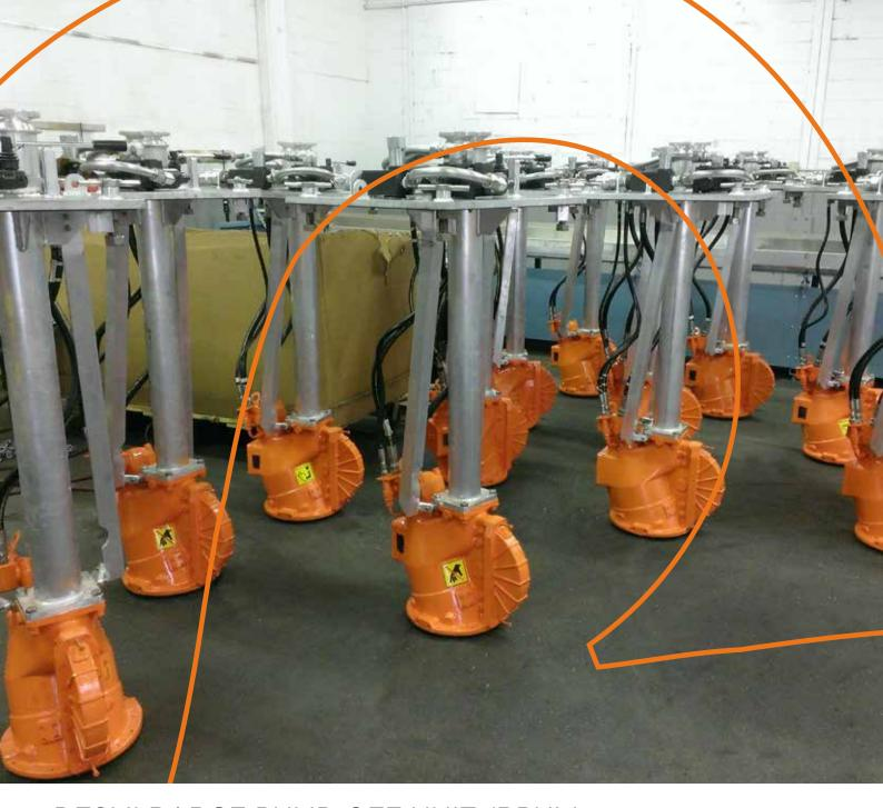
DESMI BARGE PUMP-OFF UNIT (BPU's)
